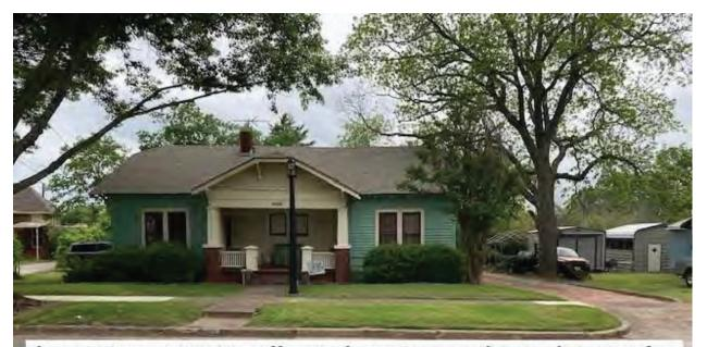
The structure at 409 W. Jefferson does not meet the requirements for a commercial establishment as it does not have a minimum side yard of 25' which is required when adjacent to a residence, in this case 413 W. Jefferson, on the right. The driveway also does not meet the standards for a two-way driveway (minimum width of 24') for a commercial establishment.
