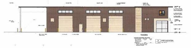
Option 2 - In this option, the building is composed of 100 percent brick on the north, east and west elevations, and metal wall panels on the south elevation. The brick color is light red.
